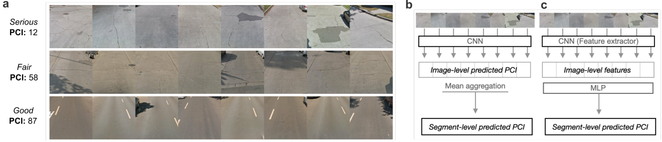
Figure 2. a) Samples of Serious, Fair and Good-rated street segments. b), c) We explore two architectures to generate segment-level predictions of pavement quality, including aggregating image-level PCI predictions ( b) and training an MLP on image-level extracted 1000-dimensional feature vectors ( c ).
