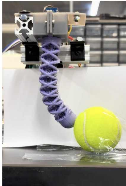
Figure 2: Probing the tennis ball during a data collection trial
